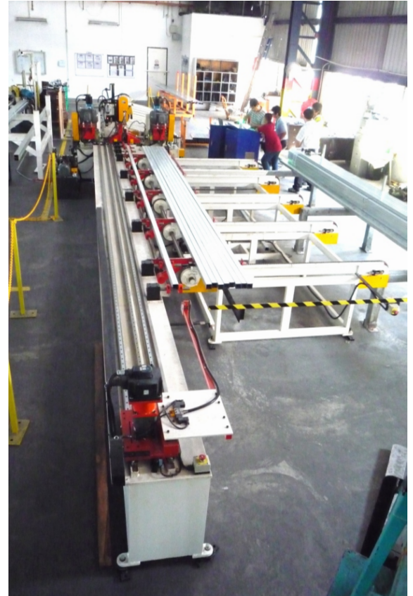
Left/Right Spindle moves UP-DOWN on the Z axis to drill the holes which are not at center of the tube.
