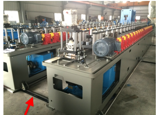
With Rail to move 2 machines to match the press
